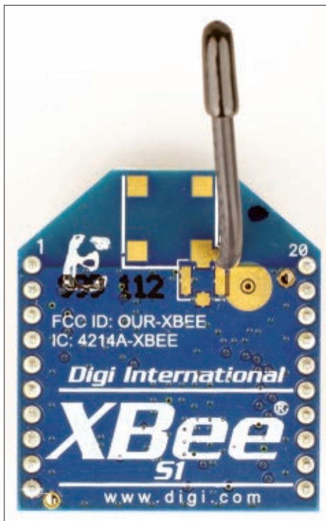
■ PHOTO 1. The FlashFly XBee radio modules operate in peer-to-peer mode under the rules of 802.15.4. This particular XBee radio module has a maximum range of 100 feet indoors and 300 feet outdoors.
