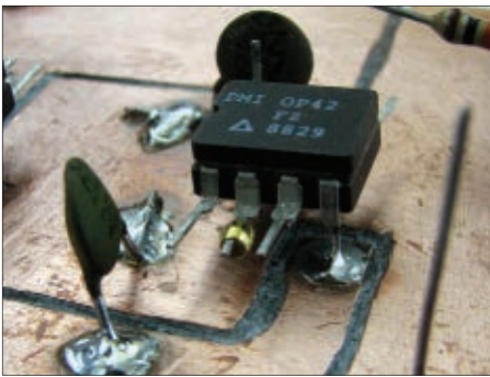
FIGURE 6A. Place a crimp bead or tube on the chip pin.
