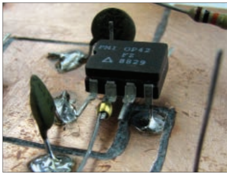
FIGURE 6B. Run the component lead inside the crimp part on top of the chip pin.
