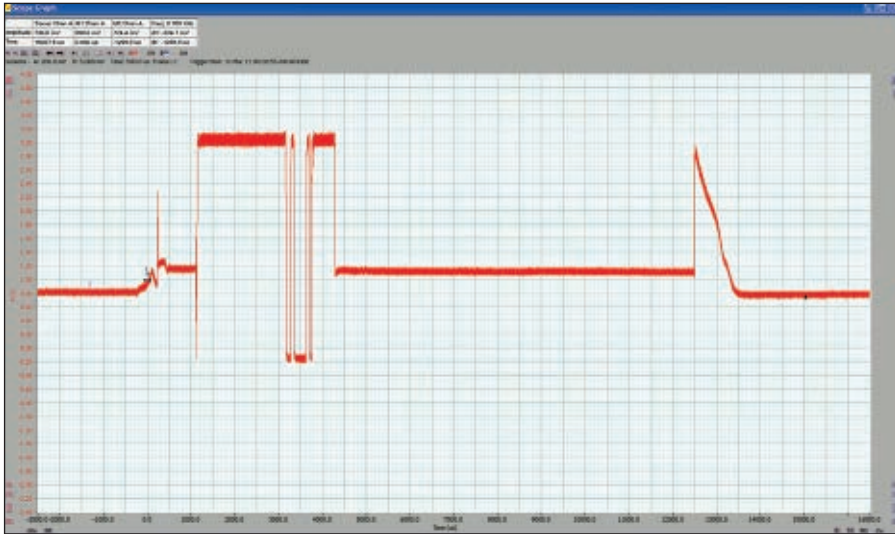
■ SCREENSHOT 1. This CleverScope capture freezes the transmitter ID bit stream. Thanks to the MCP6L04, the bits presented to the PIC24F16KA102's UART transition are between 0 and +3.0 volts.
