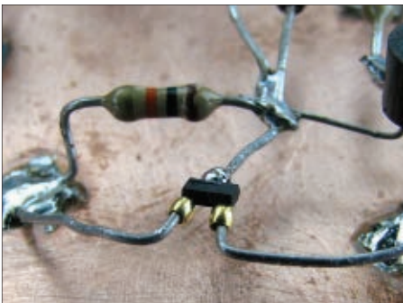
FIGURE 7A. Leads and crimp beads positioned on pins of an SOT component package.
