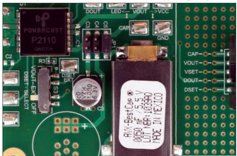
■ PHOTO 3. The high quality 50 mF capacitor stores the converted RF energy. The capacitor to its left (C3) is a test capacitor. Note the absence of receiver supporting components.
