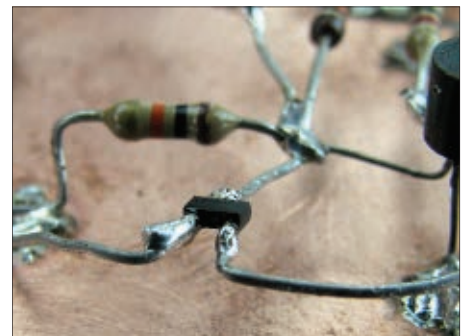
FIGURE 7C. Completed connections to the SOT package.
