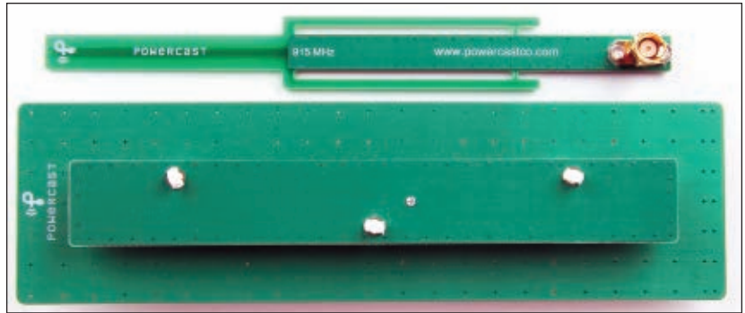
■ PHOTO 2. The dipole antenna is intended for short range power production. The larger twin-bladed patch antenna has a defined radiation pattern and offers almost 4x signal gain over the dipole.
