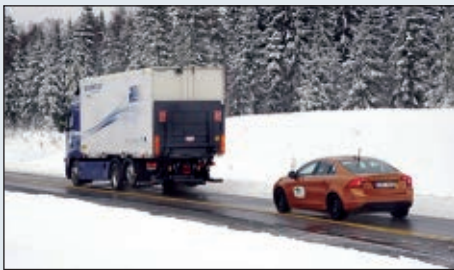
■ An autonomous Volvo follows the lead vehicle in a demonstration of the SARTRE concept.
