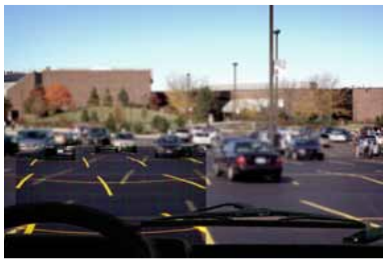
Original Camera Picture: Control the picture as texture data, by transforming YUV camera picture to RGB format
